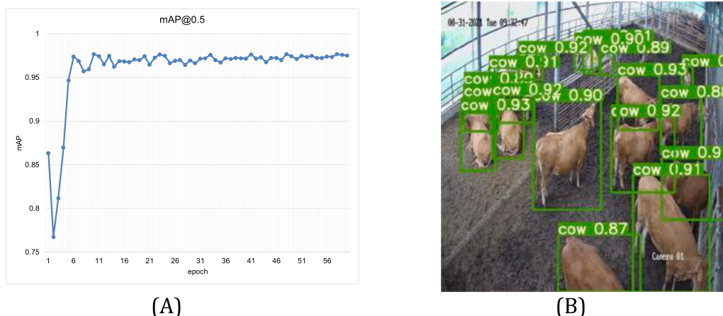
Fig. 8. Results of cattle detection based on the YOLOv5 architecture. (A) mAP curve trained with an IoU threshold of 0.5. (B) Example results of the detector on a test image.
