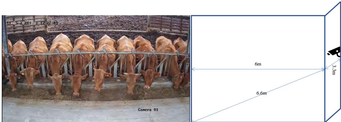
**Figure 2.** Illustration of camera installation. This figure illustrates the installation diagram of one of the cameras. We positioned a camera on the wall facing the cowshed, placing it at a height of 3.3 m above the ground and at a distance of 6 m from the cowshed.
