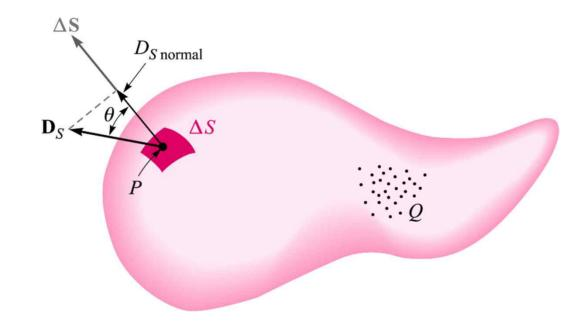
•  $\Delta S$ : incremental (surface) element of surface at P  $\Delta \vec{S} = \Delta S \vec{a}_N$  $\vec{D}_s$ : angled about  $\theta$  with  $\Delta \vec{S}$
