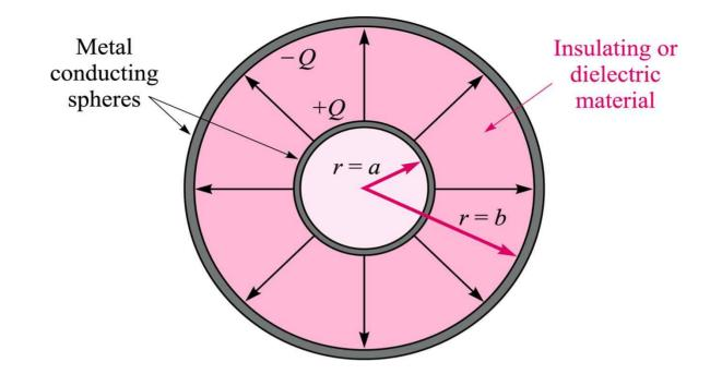
5. The inner charge, Q, induces an equal and opposite charge, -Q, on the inside surface of the outer sphere. This phenomenon is maintained for intermediate materials.
