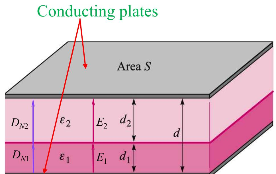
$$D_1 = D_2 \Rightarrow C = \frac{Q}{V_0} = \frac{\rho_s S}{V_0} = \frac{V_0 \cdot S \left/ \left( \frac{d_1}{\epsilon_1} + \frac{d_2}{\epsilon_2} \right) \right.}{V_0} = \frac{1}{\frac{d_1}{\epsilon_1 S} + \frac{d_2}{\epsilon_2 S}}$$
