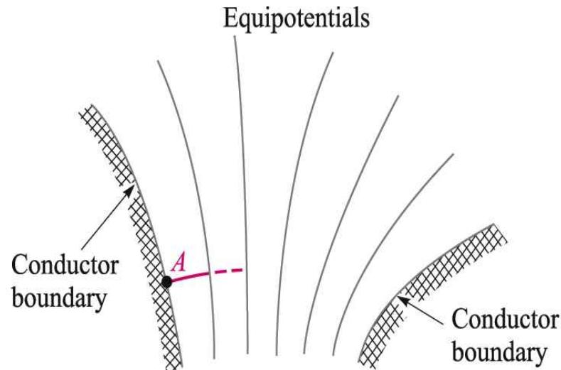
A line of electric flux density,  $\mathbf{D}$ , is then started (at point  $A$ ), and then drawn such that it crosses equipotential lines at right-angles.
