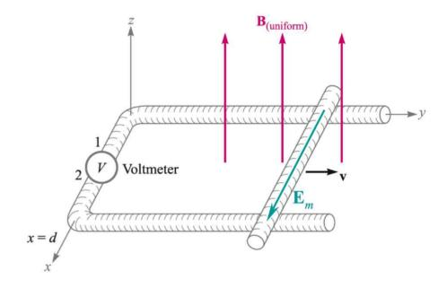
• The *motional emf* is produced by the moving conductor on uniform magnetic filed.
