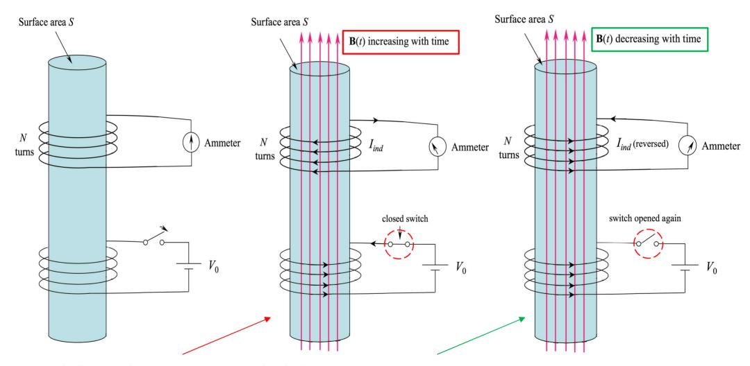
Magnetic flux density **B** generated lower circuit links the upper windings.
