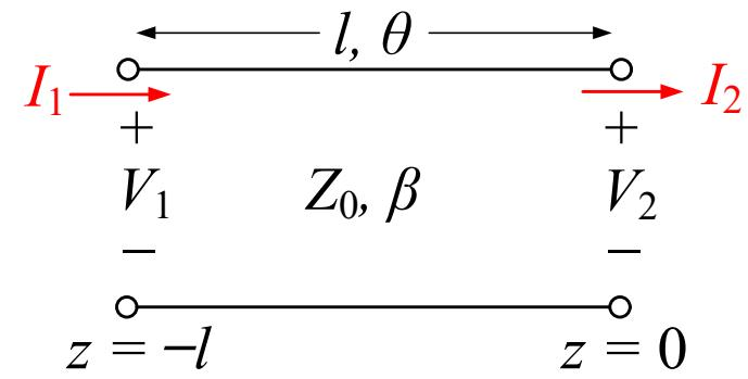
$$\begin{aligned} \Rightarrow V(z) &= V^+ e^{-\gamma z} + V^- e^{\gamma z} \\ &= \frac{1}{2} (V_2 + Z_0 I_2) e^{-\gamma z} + \frac{1}{2} (V_2 - Z_0 I_2) e^{\gamma z} \\ &= V_2 \left( \frac{e^{\gamma z} + e^{-\gamma z}}{2} \right) + I_2 Z_0 \left( \frac{e^{-\gamma z} - e^{\gamma z}}{2} \right) \\ &= V_2 \cosh \gamma z - I_2 Z_0 \sinh \gamma z \\ &= V_2 \cos \beta z - j I_2 Z_0 \sin \beta z \end{aligned}$$
