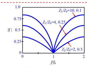
Reflection coefficient magnitude versus frequency for a single-section quarter-wave matching transformer with various load mismatches.
