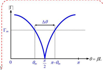
Approximate behavior of the reflection coefficient magnitude for a single-section quarter-wave transformer
