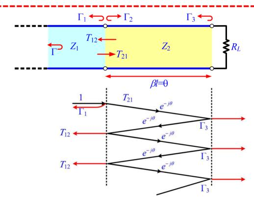
Partial reflections and transmissions on a single-section matching transformer.
