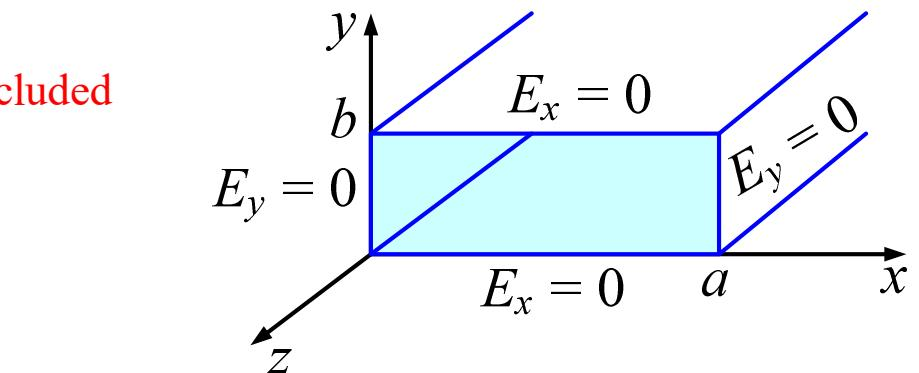
where  $\begin{cases} TE_{mn} \text{ mode : TE mode according to } m, n \\ \gamma_{mn}^2 = k_c^2 - k^2 = k_c^2 - \omega^2 \mu \epsilon, \quad \gamma_{mn} = -j\beta_{mn} \\ k_x = \frac{m\pi}{a}, \quad k_y = \frac{n\pi}{b} \\ k_c^2 = k_x^2 + k_y^2 \end{cases}$
