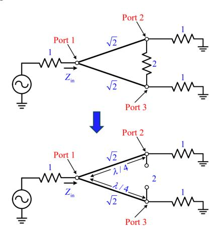
**Example:** Design an equal-split Wilkinson power divider for a 50  $\Omega$  system impedance at frequency  $f_0 = 2$  GHz, and plot the return loss  $(S_{11})$ , insertion loss  $(S_{21} = S_{31})$ , and isolation  $(S_{23} = S_{32})$  according to frequency range from 0 GHz to 4 GHz.
