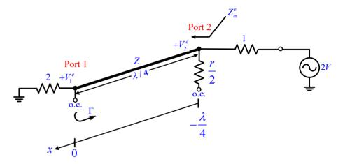
• Reflection coefficient ( $\Gamma$ ) seen at port 1, looking toward termination resistor of normalized value 2:
