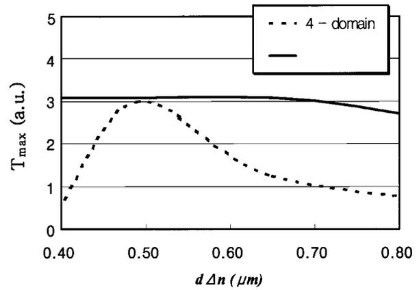
FIG. 5. Comparison of  $d\Delta n$ -dependent transmission between vertical-field driven single domain and in-plane driven VA cells.
