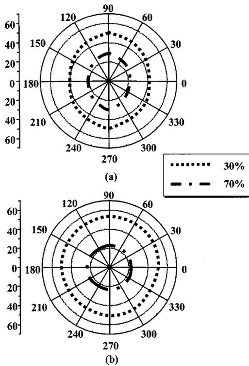
FIG. 6. The dependence of brightness of (a) 2- and (b) 4-domain VA cells in the white state on viewing angle.
