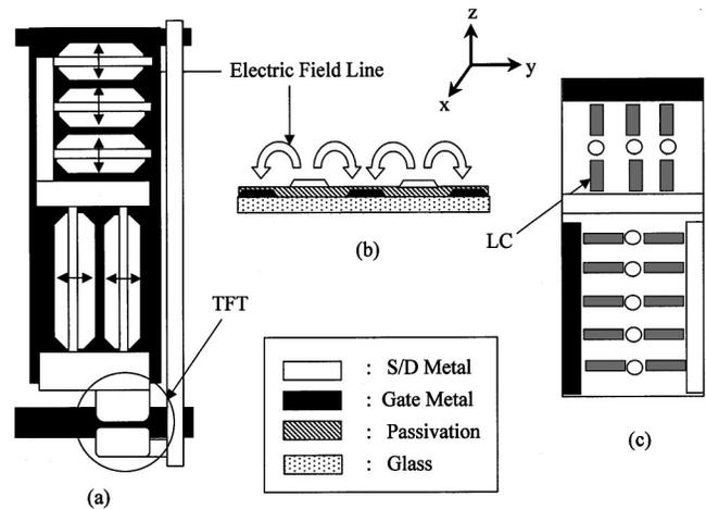
FIG. 2. (a) The array structure of the 4-domain VA cell with electric field lines, (b) cross-section view of one pixel, and (c) top view of molecular director configuration of the midplane in the on state.
