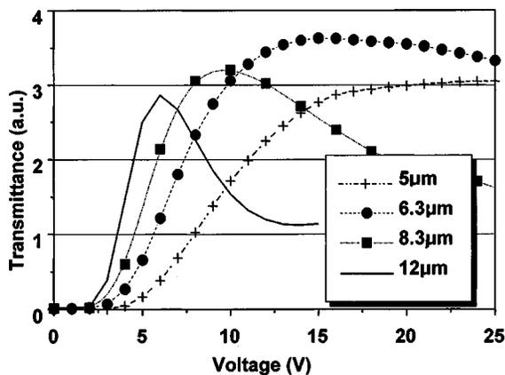
FIG. 4. The voltage dependent transmittance curves for several cells.
