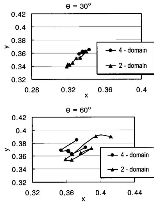
FIG. 8. The dependence of white color chromaticity at two fixed polar angles,  $30^\circ$  and  $60^\circ$  on viewing angle.
