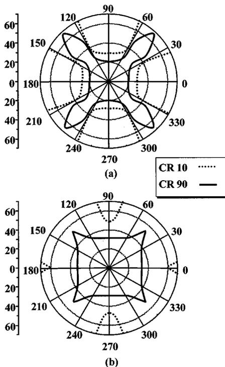
FIG. 7. The isocontrast curve (a) without and (b) with optical compensation film.
