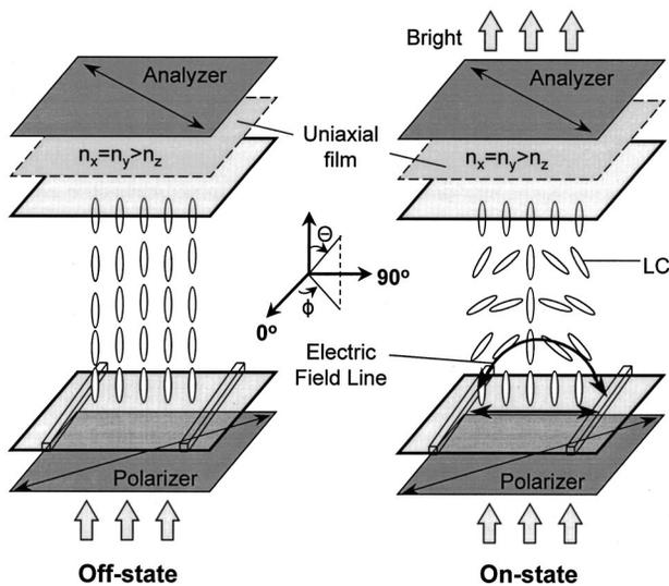
FIG. 1. The cell structures of the off and on states driven by in-plane field.
