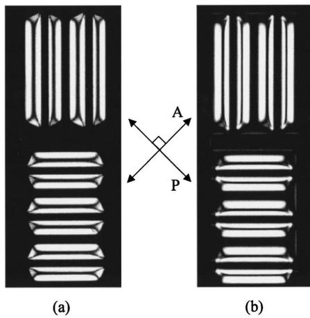
FIG. 3. A photo of one pixel with (a) low and (b) high-applied voltages in the 4-domain VA cell. P and A represent polarizer and analyzer, respectively.
