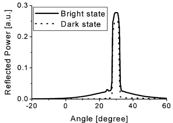
Fig. 7. Measured viewing-angle-dependent reflectance of a half-wave VA cell. The maximum contrast ratio is 24:1.
