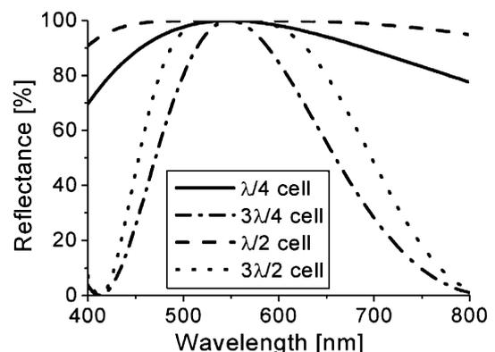
Fig. 4. Calculated reflectance of the optimized bright states with the retardation of a cell as a parameter.
