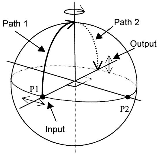
Fig. 2. Poincaré sphere representation of the polarization path of the dark state in a quarter-wave and a half-wave reflective cell.
