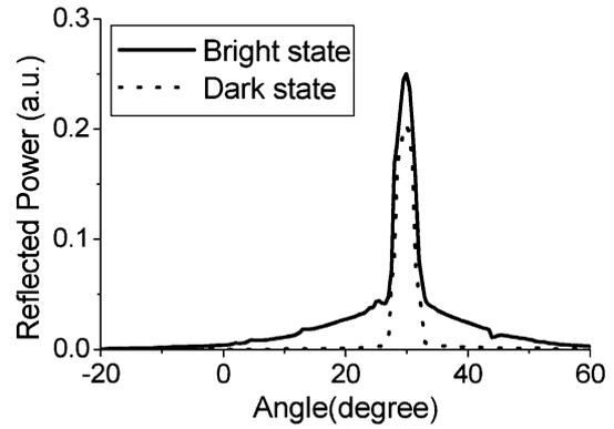
Fig. 6. Measured viewing-angle-dependent reflectance of a half-wave AFLC cell. The maximum contrast ratio is 20:1.
