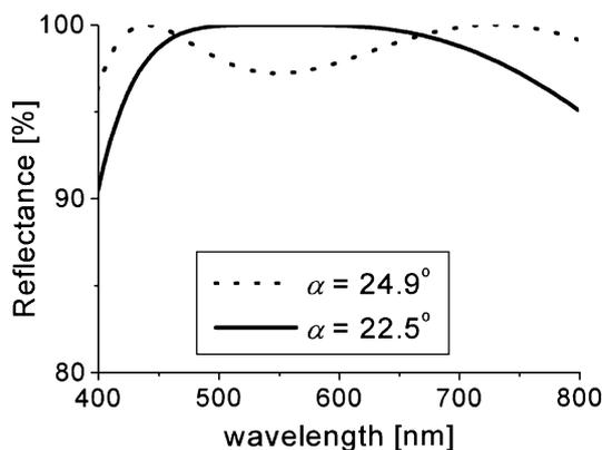
Fig. 5. The reflection spectra in the bright state. (a) an AFLC cell ( $\alpha = 24.9^\circ$ ), (b) a original design ( $\alpha = 22.5^\circ$ ).
