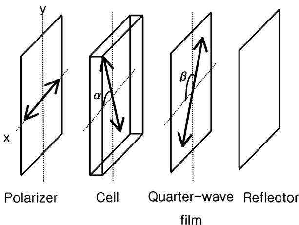
Fig. 1. Optical geometry of a single polarizer mode reflective cell.
