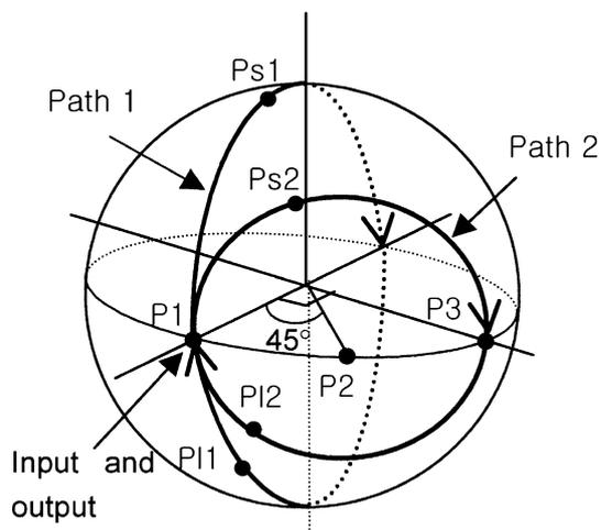
Fig. 3. Poincaré sphere representation of the polarization path of the bright state in a quarter-wave and a half-wave reflective cell.
