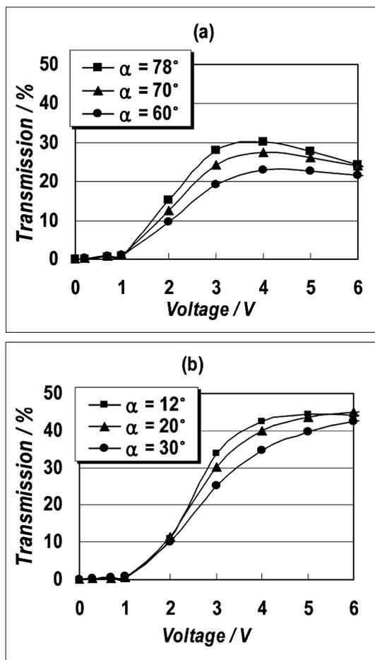
Fig. 2. The calculated result of voltage-dependent transmittance depending on rubbing direction in the FFS mode using (a) positive and (b) negative LCs.
