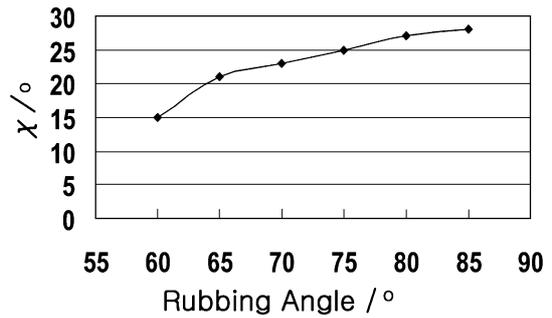
Fig. 5. The degree of rotation of the LC director above the center of electrodes dependent on rubbing angle when the operational voltage is applied.
