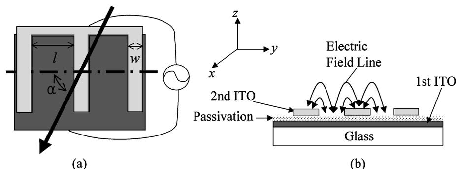
Fig. 1. Schematic diagrams of the cell structure with field lines in the FFS cell. (a) top view and (b) side view of electrodes.
