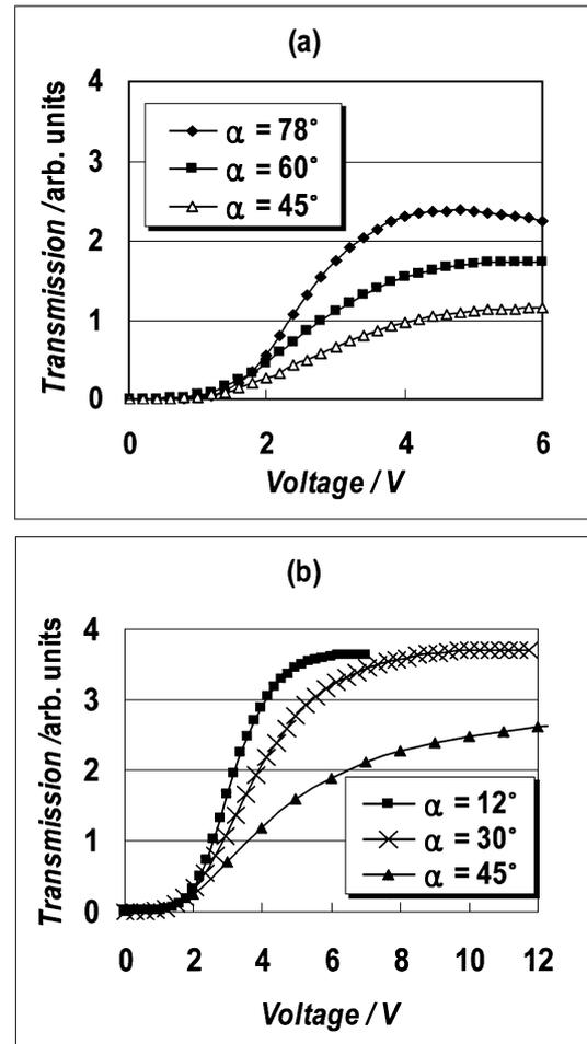
Fig. 3. The experimental result of voltage-dependent transmittance depending on rubbing direction in the FFS mode using (a) positive and (b) negative LCs.
