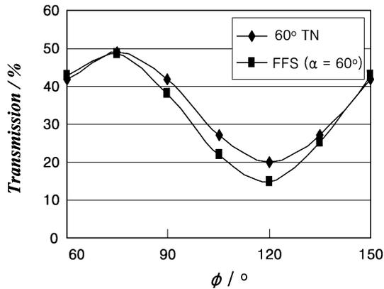
Fig. 6. Comparison of light transmission to predict the LC molecular orientation near the edge of a second electrode as a function of the optic axis of the crossed polarizers between 60° twisted TN cell and 60° rubbed FFS cell.
