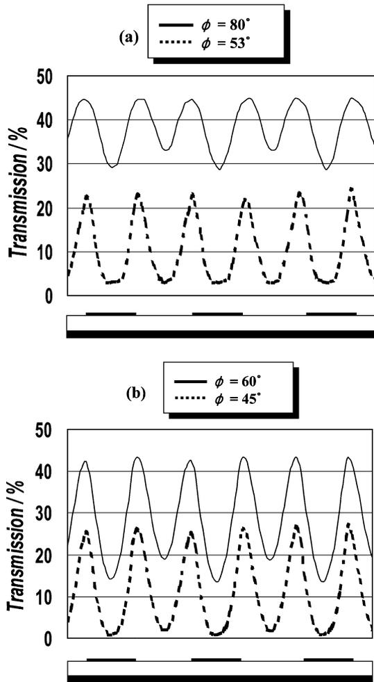
Fig. 4. The simulational result of light transmission along the y axis in a cell when operating voltage is applied and the optic axis of crossed polarizers ( $\phi$ ) is rotated to obtain the lowest transmission above the center of electrodes for (a)  $\alpha = 80^\circ$ , and (b)  $\alpha = 60^\circ$ .
