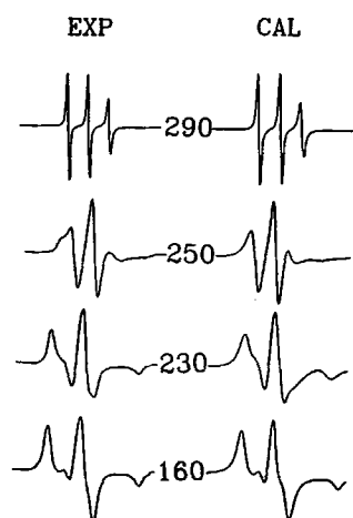
Figure 1. Experimental and calculated spectra from TPL dissolved in a mixture of 25% PVA with 75% DB by weight. The temperatures at which the spectra were observed are indicated in the center column.
