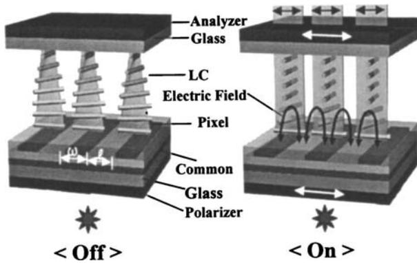
FIG. 1. Schematic of cell structure of the F-TN cell in the off and on states using a LC with negative dielectric anisotropy.
