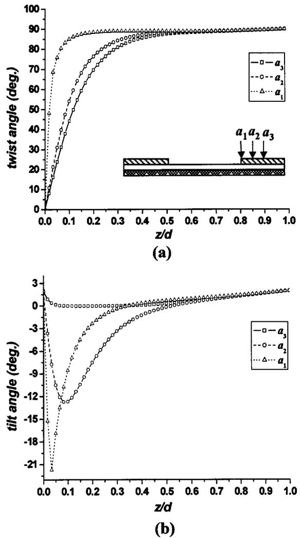
FIG. 5. Director profile of (a) twist and (b) tilt angles at three different electrode positions.
