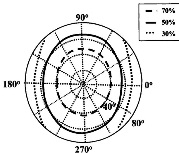
FIG. 10. Isoluminance curve for F-TN cells when the transmittance at normal direction is at a maximum.
