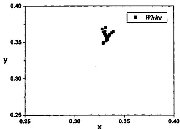
FIG. 8. Viewing angle dependence of white chromaticity up to a polar angle of  $\pm 60^\circ$  in four azimuthal directions including the horizontal, vertical and two diagonal directions.
