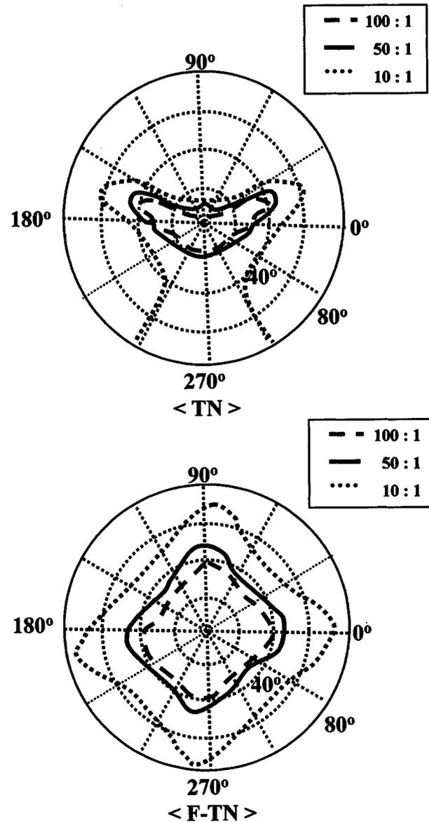
FIG. 7. Isocontrast curve for the TN and the F-TN cells at wavelength of 550 nm.
