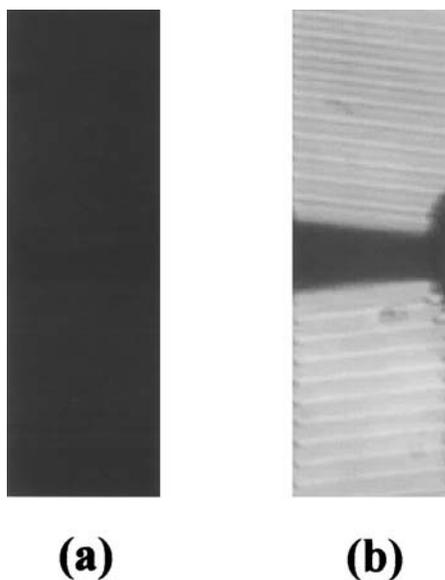
FIG. 9. Optical microphotograph of the F-TN cell in off and on states.
