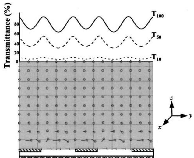
FIG. 3. Transmittance profile dependent on the electrode position at various shades of gray: low, mid- and white gray.
