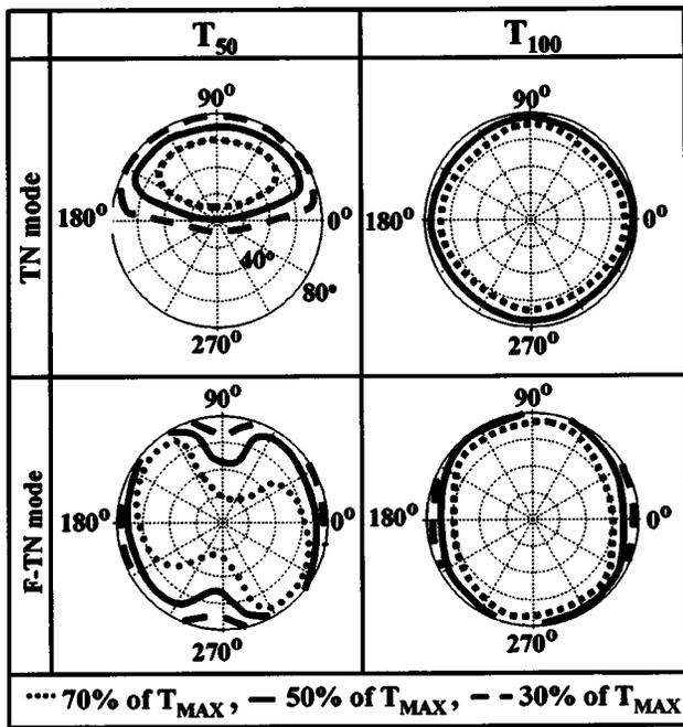
FIG. 6. Viewing angle-dependent transmittance of the TN and the F-TN cells when the transmittance at the normal direction is (a) 50% and (b) 100%.
