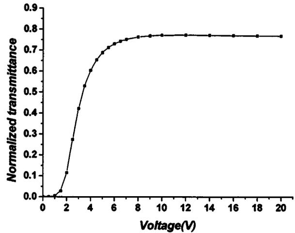
FIG. 2. Voltage-dependent transmittance curve for the F-TN cell.
