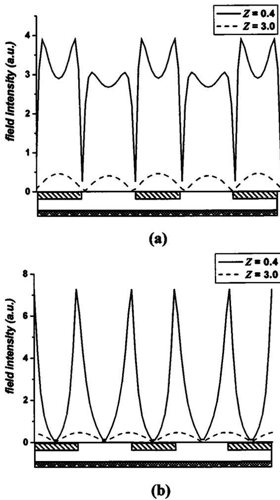
FIG. 4. Field distribution of the (a) horizontal and (b) vertical field intensity along the horizontal axis at  $z=0.4$  and  $3 \mu\text{m}$ .
