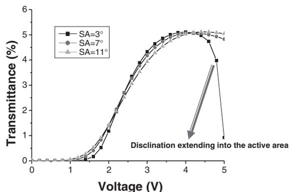
Fig. 7. Measured  $V-T$  curve in FFS mode for various slit angles.
