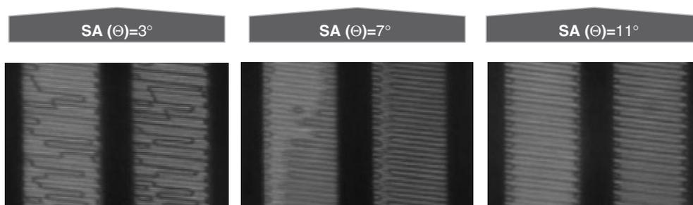
Fig. 8. Microscopy images showing how disclination lines progress with slit angle.
