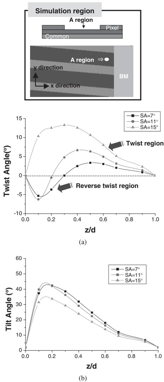
Fig. 4. LC director profile for various slit angles: (a) twist angle and (b) tilt angle.
