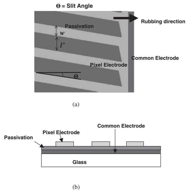
Fig. 1. Schematic diagrams of FFS cell structure: (a) top view and (b) side view of electrodes.
