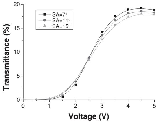
Fig. 2. Calculated  $V-T$  curve in FFS mode for various slit angles.
