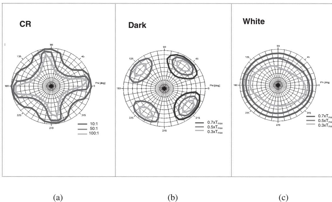
Fig. 6. Viewing angle characteristics: (a) isocontrast ratio contour, (b) isoluminance contour at  $V_{on}$  and (c) isoluminance contour at  $V_{off}$ .
