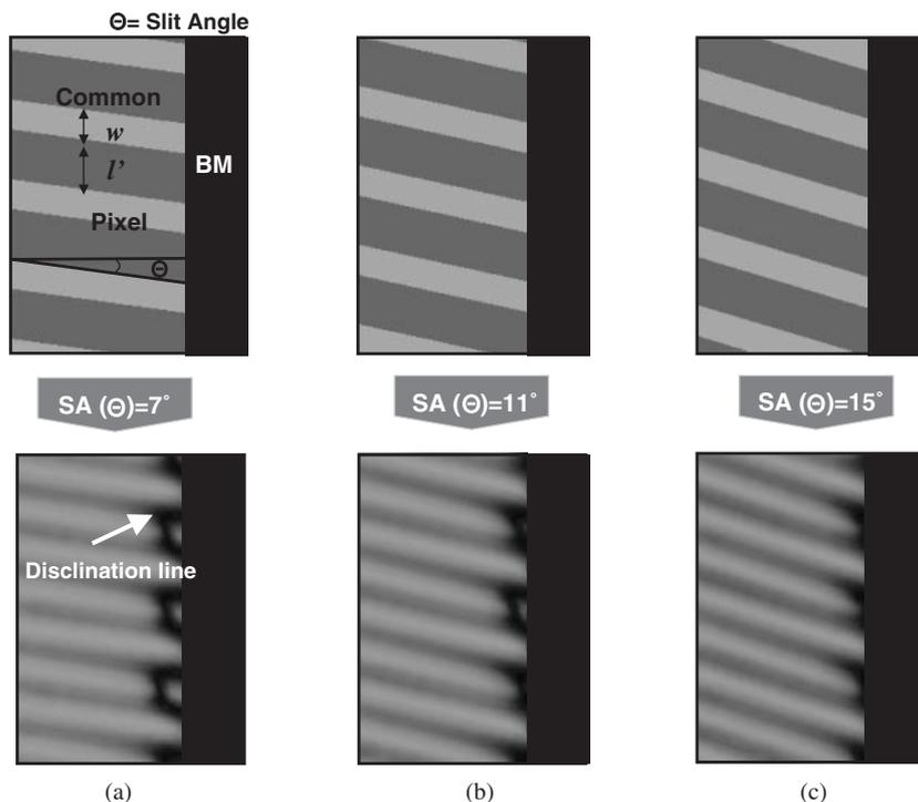
Fig. 3. Transmittance for various slit angles: (a)  $7^\circ$ , (b)  $11^\circ$  and (c)  $15^\circ$ .
