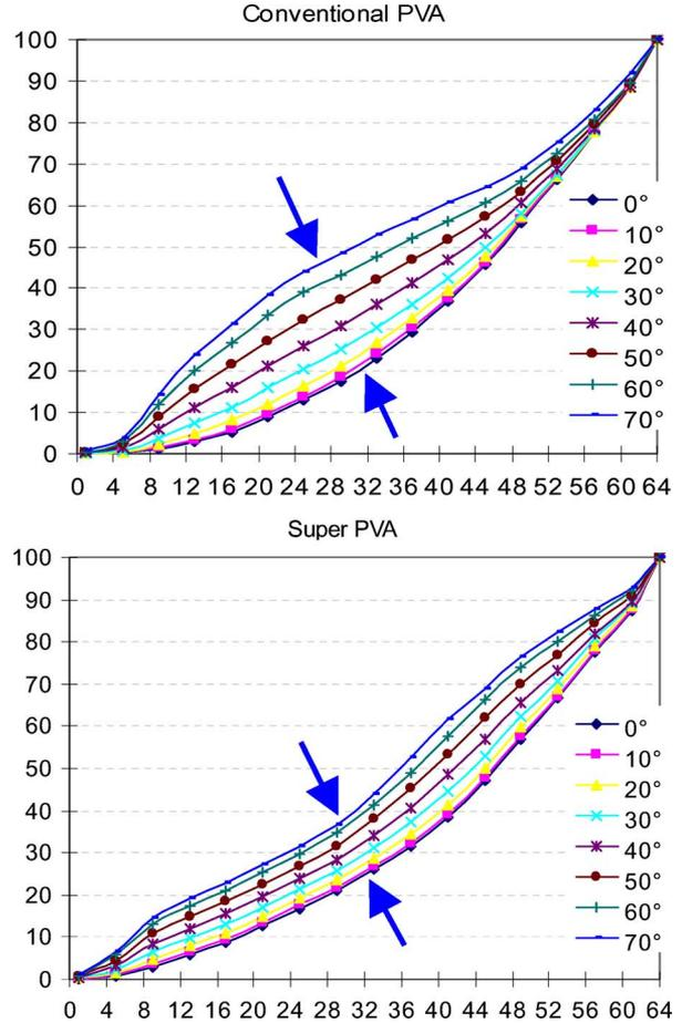
Fig. 2. Comparison of off-axis gamma between conventional PVA and S-PVA. (Permission for Reprint, courtesy Society for Information Display.)
