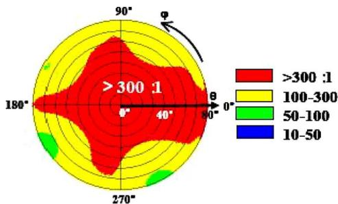
Fig. 18. Viewing angle performance of contrast ratio at 32-in LCD TV with IPS-Pro pixel structure and new compensation film. (Permission for Reprint, Courtesy Society for Information Display.)
