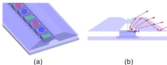
Fig. 16. Optic-structure of top emitting type LED in BOE-HYDIS 32'' AFFS-TV [24]. (a) LED array on PCB. (b) color mixing optic-system (side view).
