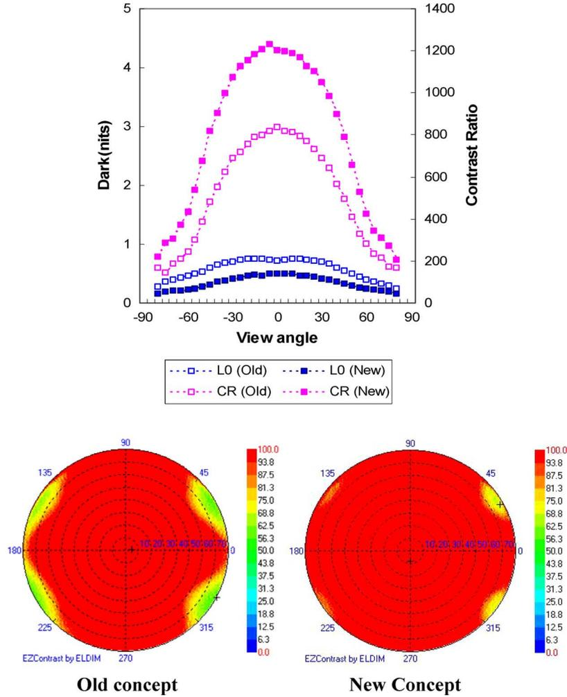
Fig. 17. The CR, dark luminance, and iso-CR contour in old and new concept polarizer in 26'' TV-AFFS.
