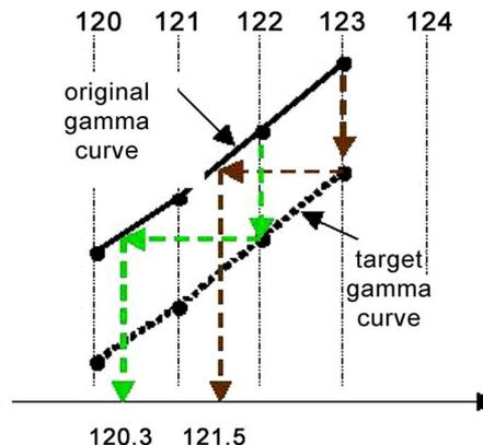
Fig. 12. Schematic diagram of gamma curve modification. (Permission for Reprint, courtesy Society for Information Display.)
