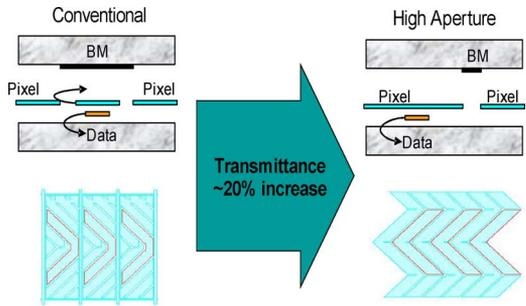
Fig. 10. Cross-section of old and new pixel structures. (Permission for Reprint, courtesy Society for Information Display.)
