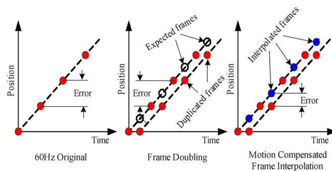
Fig. 6. Motion compensated frame interpolated driving. (Permission for Reprint, courtesy Society for Information Display.)
