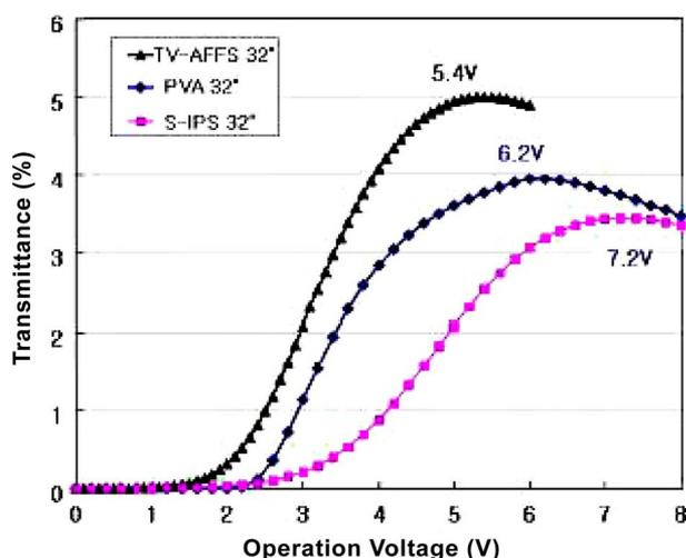
Fig. 14. Comparison of V-T Curves in FFS, S-IPS and PVA for large TV. (Permission for Reprint, courtesy Society for Information Display.)
