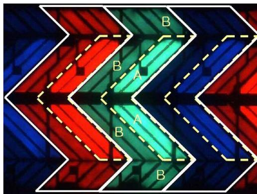
Fig. 9. A4 pixel structure of S-PVA cell. (Permission for Reprint, courtesy Society for Information Display.)
