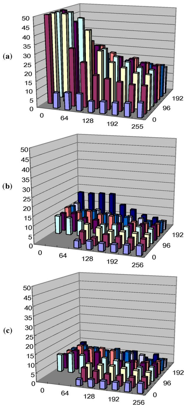
Fig. 4. Response time performance improvement by DCC techniques: (a) no DCC, (b) DCC, and (c) DCC-II in PVA panels. DCC-II accelerates the response time to less than 10 ms for all image transitions. (Permission for Reprint, courtesy Society for Information Display.)
