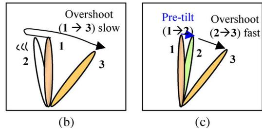
Fig. 3. Basic concept of DCC-II technology. (a) DCC-II signal and response. (b) LC action: no pre-tilt. (c) LC action: with pre-tilt. (Permission for Reprint, courtesy Society for Information Display.)
