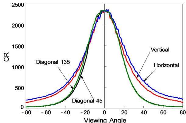
Fig. 8. New S-PVA panel contrast ratio versus viewing angle. (Permission for Reprint, courtesy Society for Information Display.)
