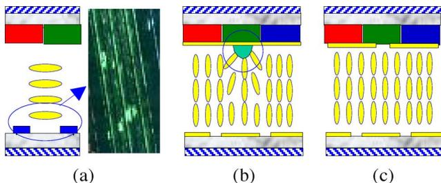
Fig. 7. Cross-sectional diagram of the various liquid crystal cell structures in the black state. (a) IPS mode. (b) MVA mode. (c) PVA mode. (Permission for Reprint, courtesy Society for Information Display.)
