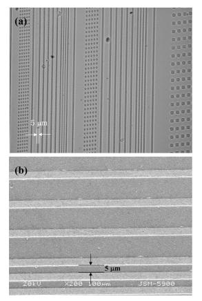
**Figure 7**. (a) Optical microscopic image and (b) scanning electron microscopic image of line-and-space patterns obtained from PI-DMNB.
