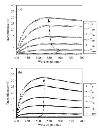
Figure 2. Wavelength dependent-transmittance in a fringe-field switching device using the (a) +LC and (b) -LC with respect to the grey level.
