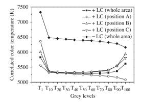
Figure 5. Correlated colour temperature of a fringe-field switching device with +LC and -LC with respect to the grey level.
