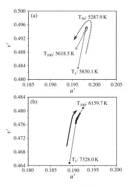
Figure 3. Colour chromaticity in u'v' coordinates of a fringe-field switching device using the (a) +LC and (b) –LC device according to the grey level.
