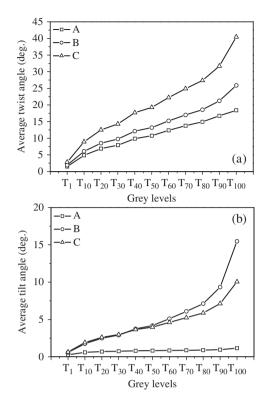
Figure 8. Average (a) twist and (b) tilt angle of liquid crystal directors at three different electrode positions.
