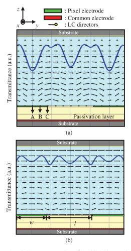
Figure 1. Cell structure and profile of liquid crystal (LC) orientation and transmittance in the white state of a fringe-field switching device when using the (a) +LC and (b) -LC.
