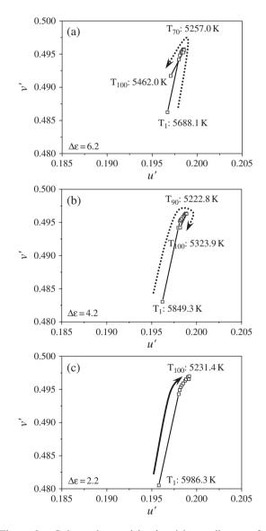
Figure 9. Colour chromaticity in u'v' coordinates of a fringe-field switching device using the +LC according to dielectric anisotropy: (a)  $\Delta \varepsilon = 6.2$ ; (b)  $\Delta \varepsilon = 4.2$ ; (c)  $\Delta \varepsilon = 2.2$ .
