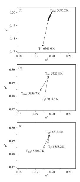
Figure 4. Colour chromaticity in u'v' coordinates of a fringe-field switching device with the +LC according to the electrode position: (a) A; (b) B; (c) C.
