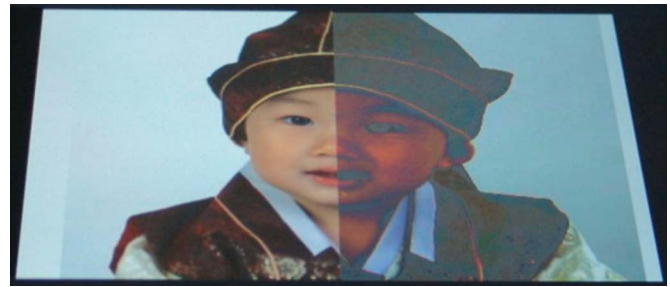
FIG. 6. (Color online) Photographs of the 19.0 in. TFT-LCD of the WV-TN without (right) and with (left) the BSF layer at a polar angle of -50^\circ .
