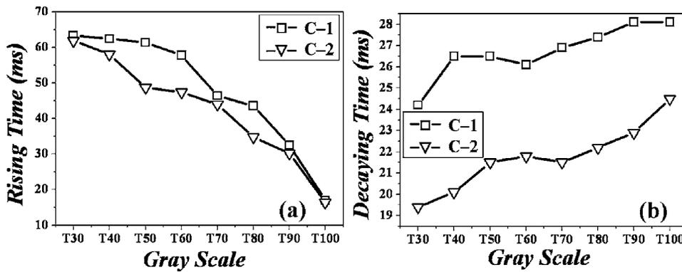
FIG. 5. Measured (a) rising and (b) decaying response times of the pure LC and CNTs-doped LC cells. The numbers in the label of the row axis show the relative transmittance with respect to the maximum transmittance at the normal direction.
