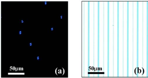
FIG. 2. (Color online) Polarization microphotographs of (a) off and (b) on states of the pure and CNT-doped IPS cells.
