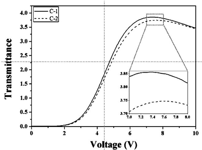
FIG. 3. Measured voltage-dependent transmittance curves of the pure and CNT-doped LC cells.
