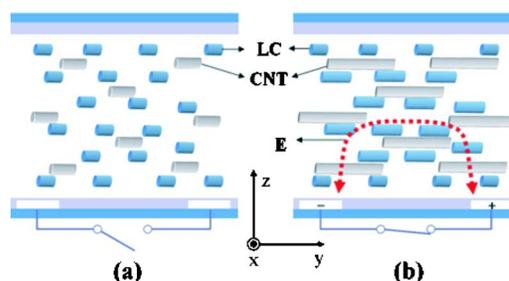
FIG. 1. (Color online) Schematic of the cell structure of the CNT-doped nematic LC cells in (a) off and (b) on states.
