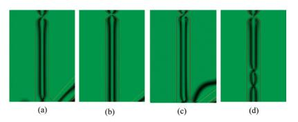
**Figure 5.** Calculated optical transmittance as a function of the length of the slit: (a) reference (20  $\mu$ m), (b) 25  $\mu$ m, (c) 30  $\mu$ m, (d) 35  $\mu$ m. (Figure appears in color online.)
