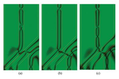
**Figure 6.** Calculated optical transmittance as a function of the width of the slit: (a) the conventional cell with  $8 \mu m$  of the slit width, (b) the proposed cell with  $8 \mu m$  of the slit width, (c) the proposed cell with  $7 \mu m$  of the slit width. (Figure appears in color online.)
