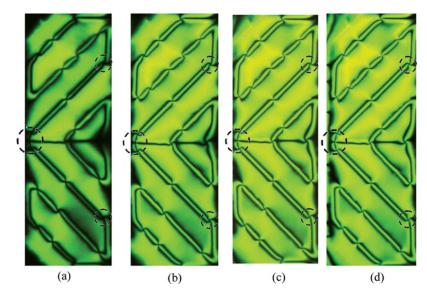
**Figure 4.** Optical Transmittance of the fabricated PVA LC cell with the defect trap structure: (a) at 4 V, (b) at 6 V, (c) at 8 V, (d) at 10 V. (Figure appears in color online.)
