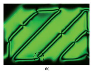
**Figure 3.** Optical transmittance of the fabricated PVA LC cell at the white state: (a) the conventional cell at 4 V, (b) the proposed cell at 4 V. (Figure appears in color online.)
