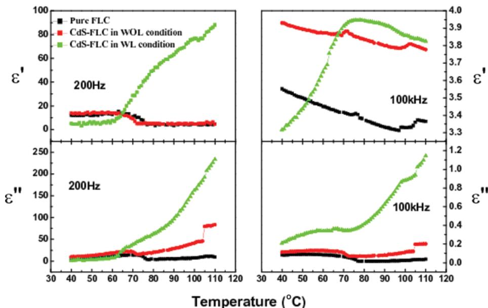
**Figure 2.** Real ( $\epsilon'(\omega)$ ) and imaginary part ( $\epsilon''(\omega)$ ) of dielectric permittivity at 200 Hz (a) and 100 kHz (b) of three samples: Pure FLC, CdS-FLC in absence of light (WOL condition), CdS-FLC in presence of light (WL condition).
