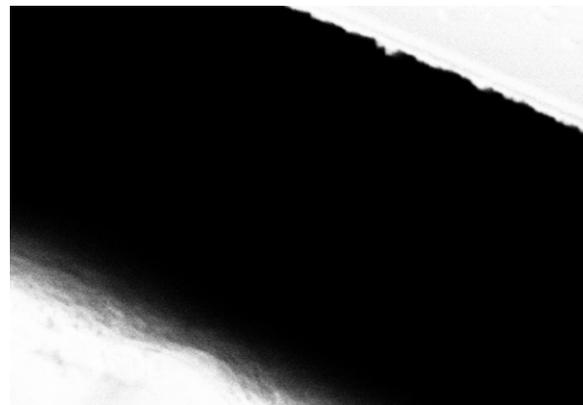
**Figure 7.** Vertical SEM image of 20 000 times magnified assembled cell having gap 3.5  $\mu\text{m}$ . The dark image indicates no polymer network in the bulk of LC layer.
