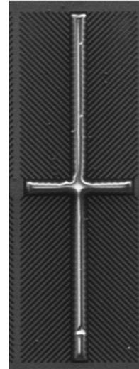
**Figure 1.** Micro-slit structure of PS-VA mode.
