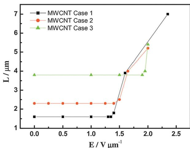
**Fig. 3** (Color online) MWCNT cluster length variation with varying electric field in a few representative cases.
