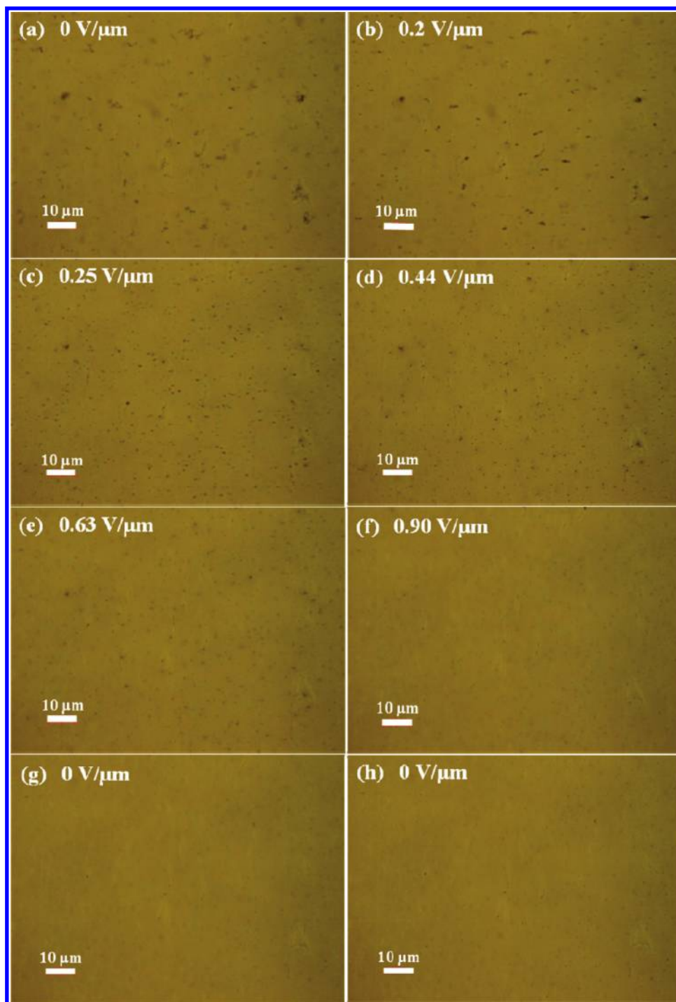
Figure 1. (a–h) Optical microphotographs of CNT-LC cell with respect to electric field (0, 0.20, 0.25, 0.44, 0.63, 0.90, and 0 V/ \mu\text{m} ) viewed through a linear polarizer, (g) optical image right after field is removed, and (h) optical image after field is removed and the cell is maintained for 48 h.
