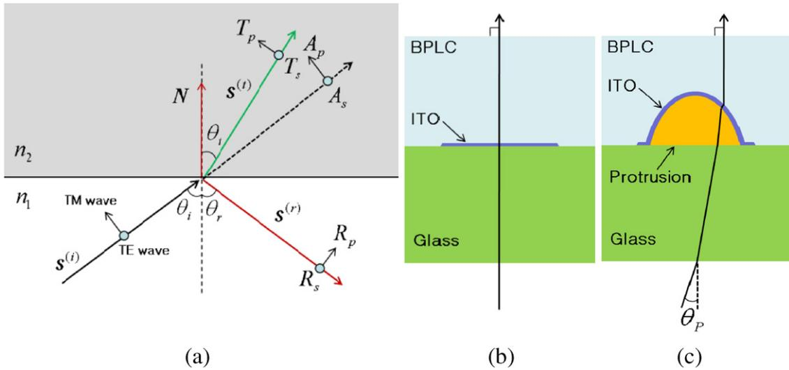
**Figure 5.** Vector expression of (a) a relatively refracted angle to the incidence direction and full path of light in (b) the conventional normal cell and (c) the protruded electrode cell.
