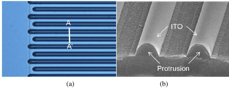
**Figure 1.** Cell structure with protruded electrodes: (a) top view of microscopic image and (b) cross-sectional view taken by a scanning electron microscope (SEM) in the A–A' direction.
