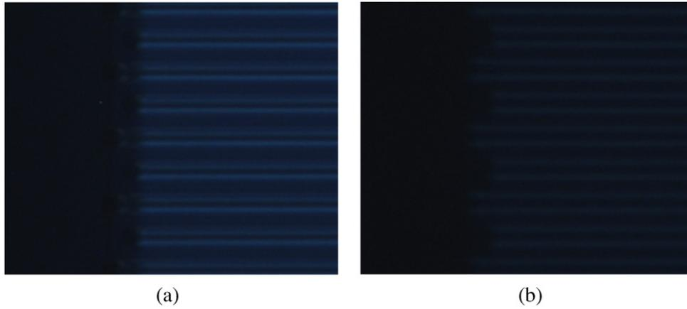
**Figure 3.** Light intensity distribution of the IPS cell when the electrode pattern direction is at 45° with respect to the crossed polarizer: (a) protruded electrode cell, (b) normal electrode cell.
