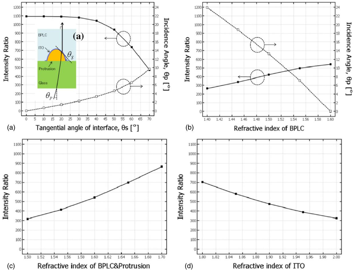
**Figure 7.** Intensity ratio curves according to (a) the tangential angle of protrusion interface,  $\theta_s$  and variation of refractive index of (b) BPLC, (c) BPLC and protrusion (matched), and (d) ITO at  $70^\circ$  of tangential angle.
