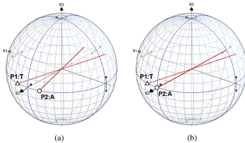
**Figure 6.** Change in the effective angle between two polarizers (P1:T—transmittance axes of the polarizer and P2:A—absorption axes of the analyser) in the case of (a) oblique incidence to the crossed polarizer and (b) the sloped interface.
