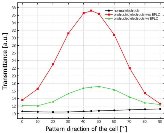
**Figure 4.** Light leakage according to the pattern direction of the cell with crossed polarizer for three different cells: normal, protruded electrode without BPLC (w/o BPLC) and protruded electrode with BPLC (w/ BPLC).
