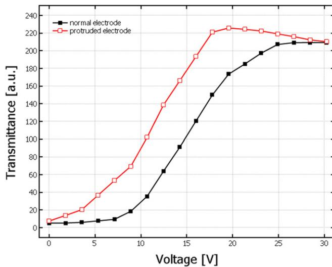
**Figure 2.** Voltage-dependent transmittance characteristics for the IPS cells with protruded and normal electrodes.
