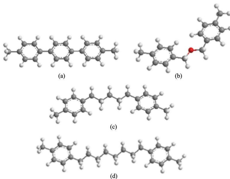
**Figure 6.** (colour online) Diamine structures of each polyimide alignment materials (white balls: hydrogen, grey balls: carbon, red ball: oxide). (a) PI-A, (b) PI-B, (c) PI-C, (d) PI-D.
