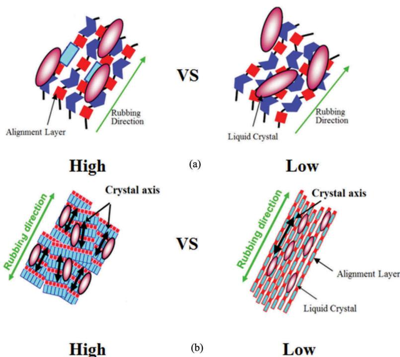
**Figure 5.** (colour online) Schematic concepts of LC director alignment depending on structures of the alignment layers: (a) the polymer flexibility with high and low degree and (b) the polymer crystallinity with high and low degree. The layer with structures of high flexibility and low crystallinity exhibits better LC alignment along the rubbing direction.
