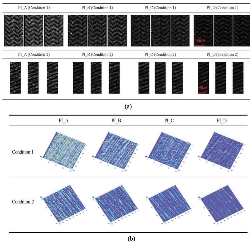
**Figure 7.** (colour online) (a) Captured images of the light leakage and (b) converted digital three-dimensional distribution images of the rubbed textures in each PI. The measured sizes for condition I and II are  $300\ \mu\text{m} \times 450\ \mu\text{m}$  and  $70\ \mu\text{m} \times 200\ \mu\text{m}$ , respectively.
