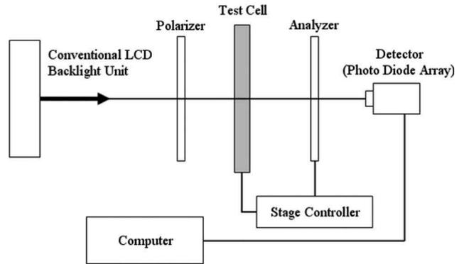
Figure 4. A brief schematic system for measuring transmittance in black state of IPS cells.
