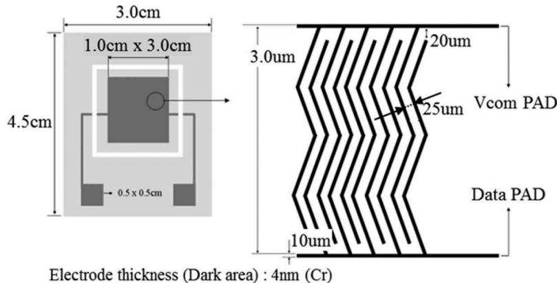
Figure 3. Schematic cell structure of the IPS test cell used for measuring light leakage.
