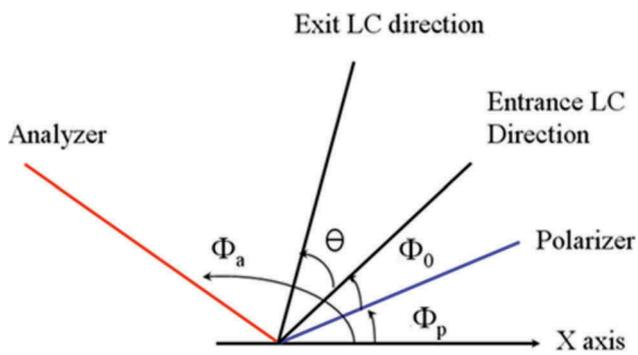
**Figure 2.** (colour online) Definition of angles for polariser, analyser, and, entrance and exit LC direction with respect to X-axis.
