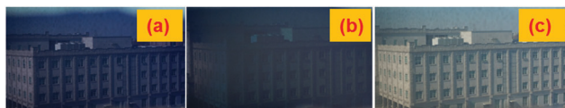
Fig. 7 The transparency of various states of DFCLC with 2 wt% dye: (a) planar state, (b) focal conic state, and (c) homeotropic state.
