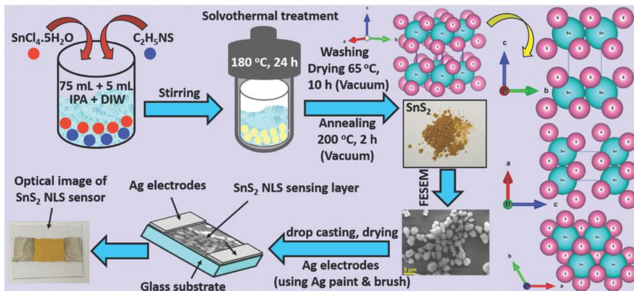
Scheme 1 Schematic representations of SnS 2 NLS synthesis, crystal structure visualization, and sensor device fabrication.
