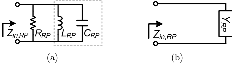
Figure 3.10: Lumped element NGD circuit in 1-port reflective configuration: (a) reflective-parallel structure and (b) its equivalent admittance representation.
