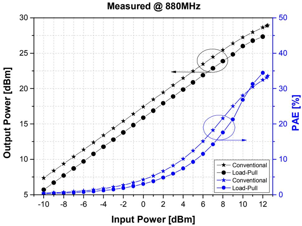
Fig. 5.3. Compare the result between conventional PA with load-pull measurement result.
