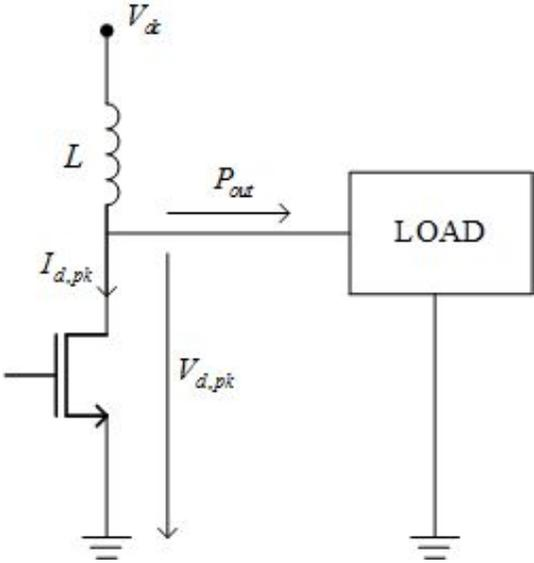
Fig. 2.1. Power output capability in RF power amplifiers.
