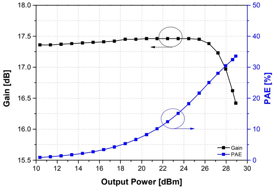
Fig. 5.2. Conventional PA measurement result.
