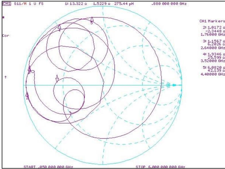
Fig. 5.7. Load impedance circle measurement result of proposed DGS output matching network.
