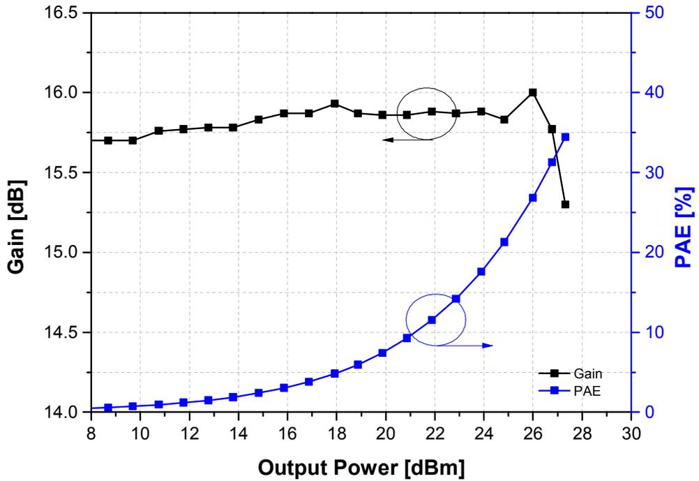
Fig. 4.5. Result of the load pull measurement.
