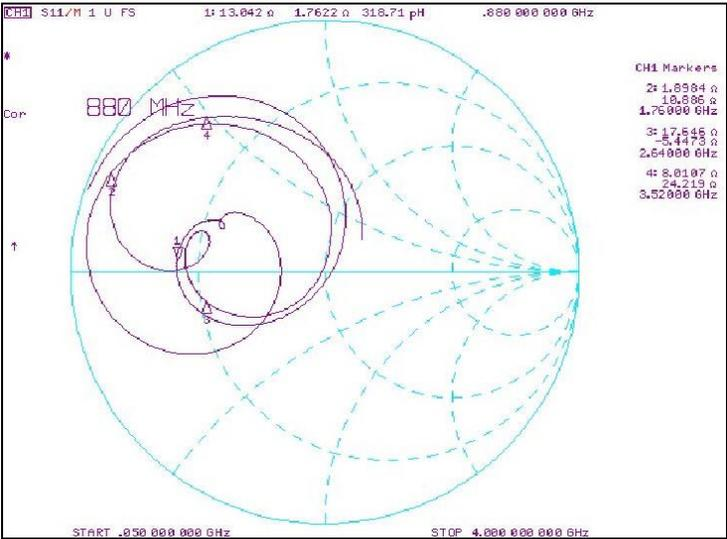
Fig. 4.21. Load impedance circle of measured result.
