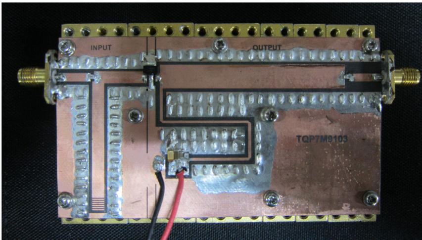
Fig. 5.1. Photograph of fabricated power amplifier.
