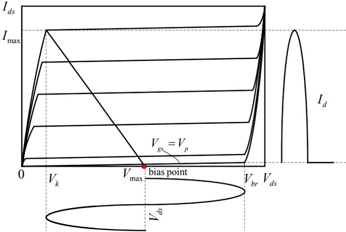
Fig. 2.3. Class B bias condition and output waveform.
