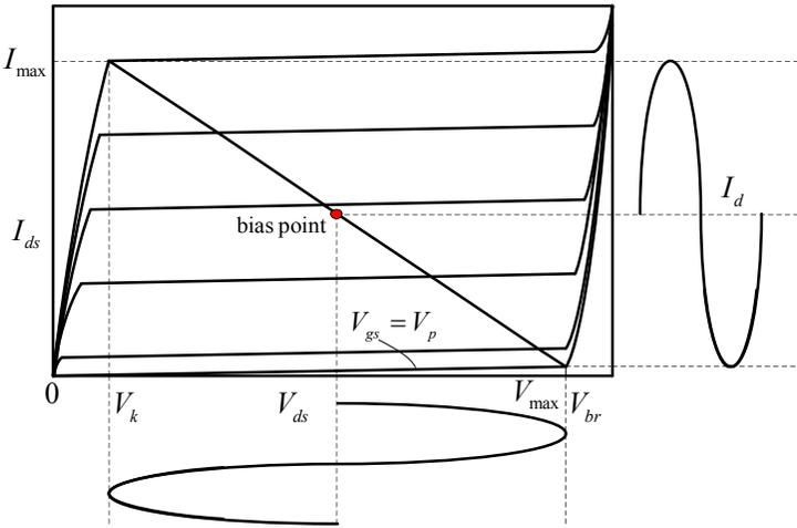
Fig. 2.2. Class A bias condition and output waveform.
