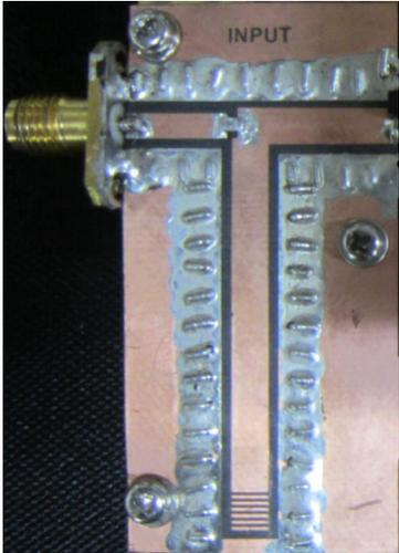
Fig. 4.12. Photograph of the fabricated input matching circuit for 880MHz.
