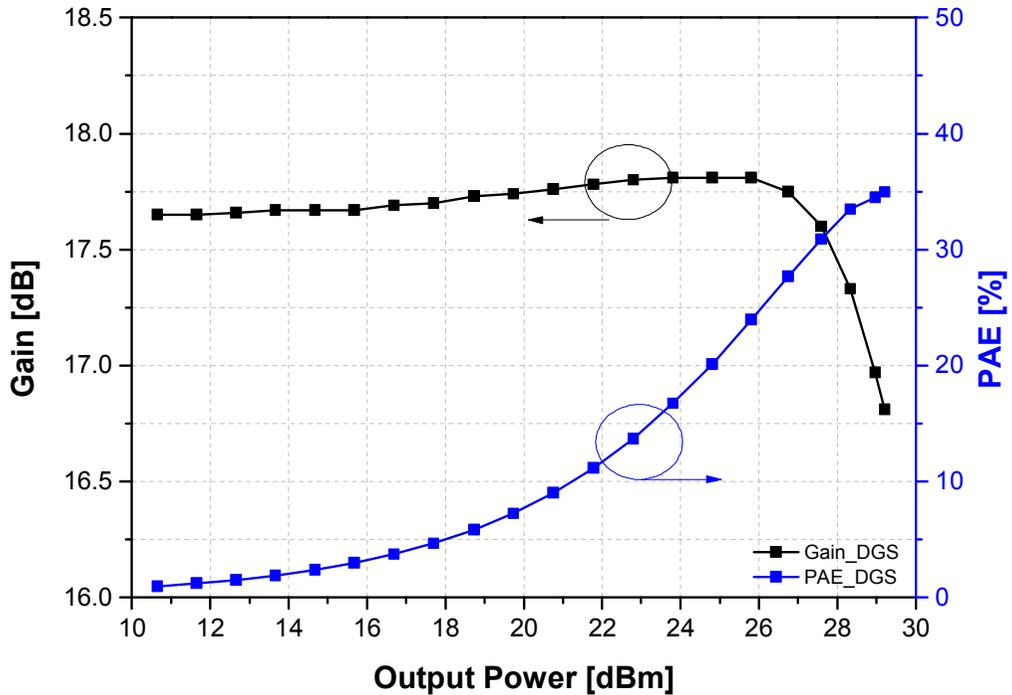
Fig. 5.10. DGS power amplifier measurement result.
