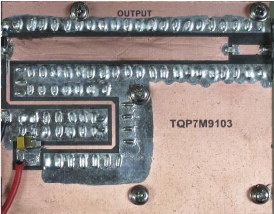
Fig. 4.20. Photograph of the fabricated output matching circuit for 880MHz.
