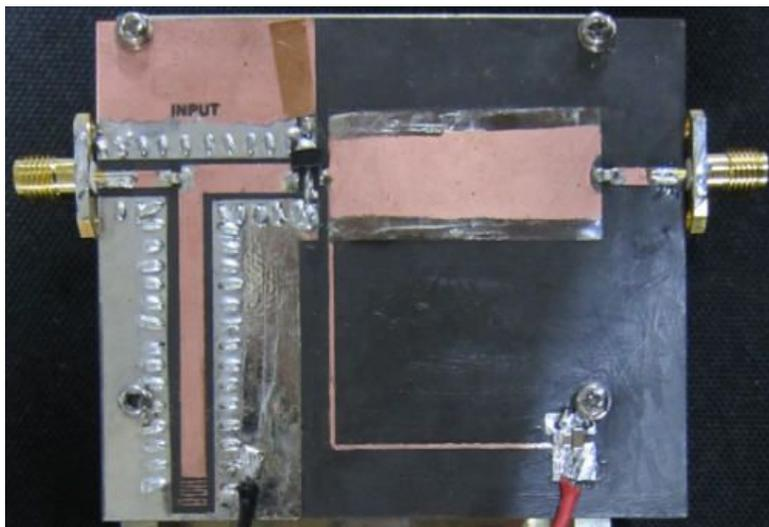
Fig. 5.9. Photograph of fabricated DGS power amplifier.
