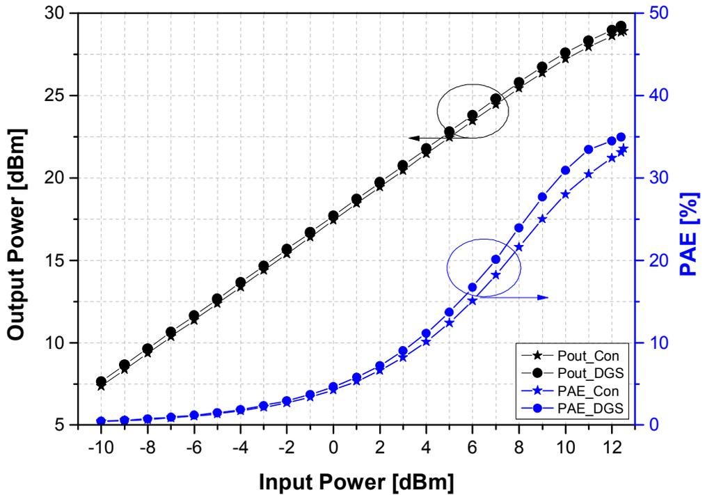
Fig. 5.11. Compare the measurement result between conventional and DGS power amplifier.
