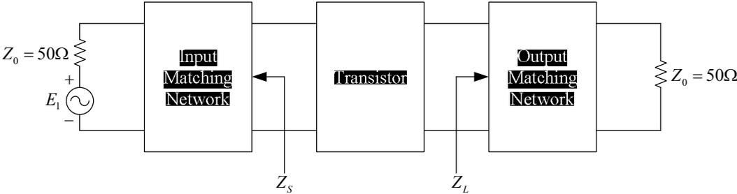
Fig. 2.6. Block diagram of a amplifier.
