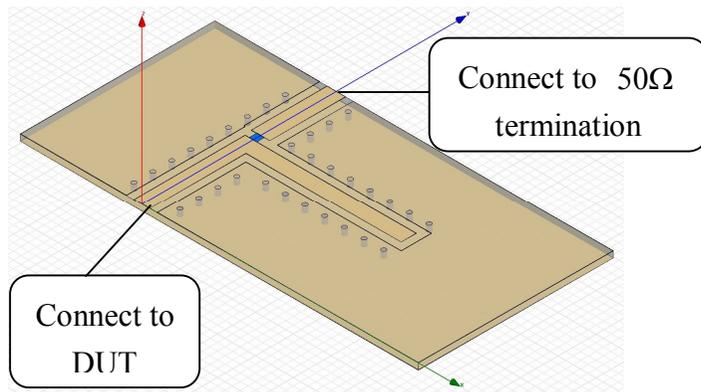
Fig. 4.10. Layout of input matching network.
