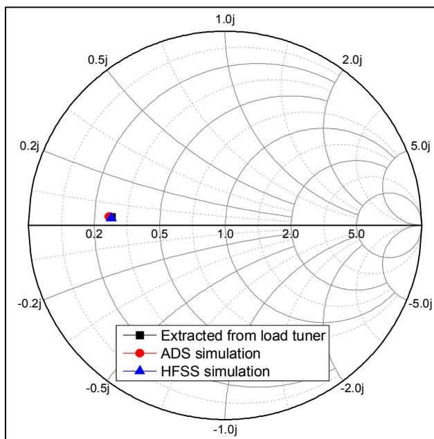
Fig. 4.19. Load impedance of tuner, ADS, and HFSS circle.
