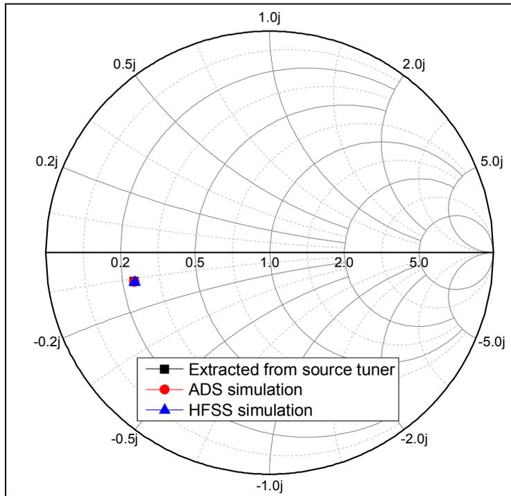
Fig. 4.11. Source impedance extracted from tuner, ADS and HFSS.
