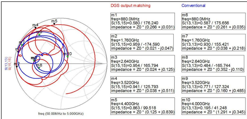
Fig. 5.8. Load impedance circle of the Measurement result between conventional and proposed DGS output matching network.
