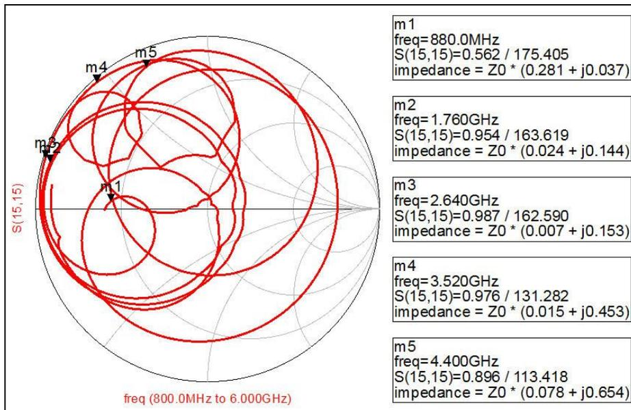
Fig. 5.5. HFSS simulated load impedance circle of proposed DGS output matching.
