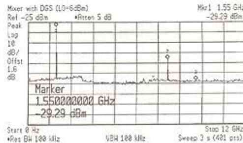
Fig. 6. The frequency characteristics of drain mixer using DGS \lambda/4 bias line. (@ P_{LO} =6dBm, P_{RF} =-30dBm)
