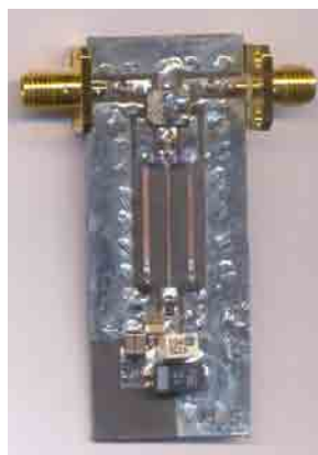
Fig. 7. The photograph of the fabricated a novel low phase deviation variable attenuator.
