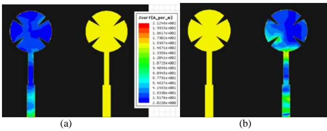
Figure 6: Current Density for both the elements of the proposed MIMO antenna.
