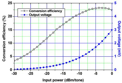
Fig. 4. Measurement results of conversion efficiency and output voltage of proposed dual band RF energy harvesting circuit in condition of  $R_L = 20 \text{ K}\Omega$ .
