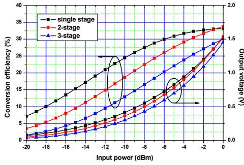
Fig. 2. Simulation results of conversion efficiency and output voltage according to number of stages in condition of  $R_L = 5 \text{ K}\Omega$ .
