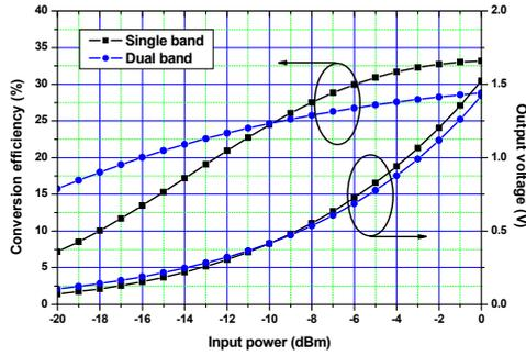
Fig. 3. Simulation results of conversion efficiency and output voltage according to single band (2.44 GHz) and dual band (0.88/2.44 GHz) with in condition of  $R_L = 5 \text{ K}\Omega$ .
