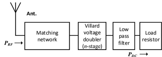
Fig. 1. Block diagram of proposed RF energy harvesting circuit.
