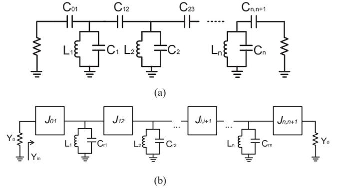
Fig. 3 Structures of proposed CMOS BPF using: (a) lumped elements and (b)  $J$ -inverters.
