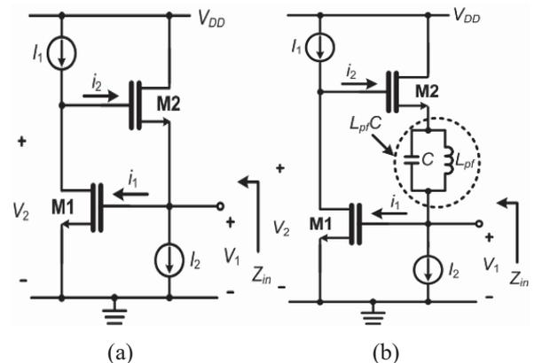
Fig. 1 (a) Conventional GAI and (b) high Q active inductor using LC parallel resonator.
