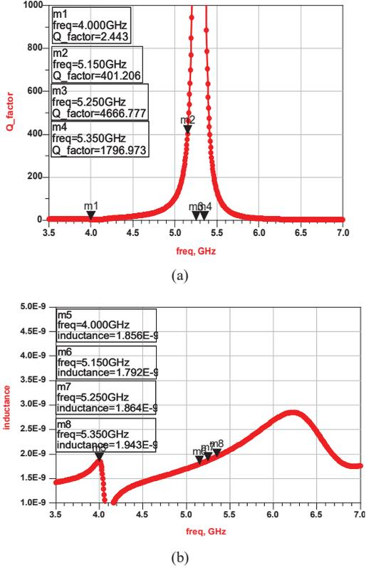
Fig. 2 (a) Q-factor and (b) inductance characteristics of active inductor using feedback parallel resonator
