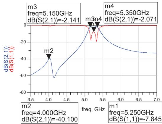
Fig. 4 Simulation result of proposed BPF
