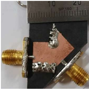
Fig. 9. Photograph of fabricated quarter-mode SIW BPF with square/triangle cavities.
