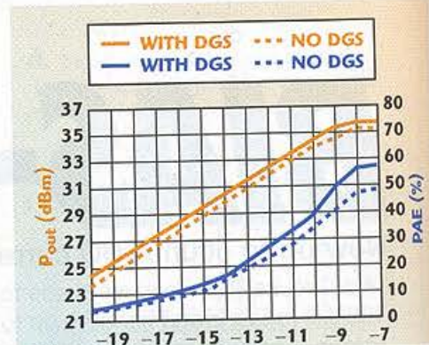
▲ Fig. 8 Measured P_{out} and PAE of the power amplifiers with and without DGS bias lines.
