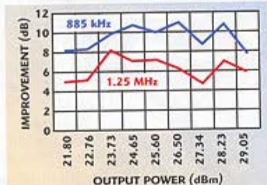
▲ Fig. 11 HPA ACPR improvement as a function of output power for a CDMA signal.
