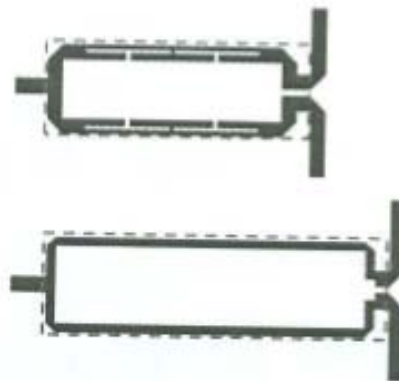
Fig. 5. Layout of power dividers using DMS microstrip line (upper) and normal microstrip line (lower)
