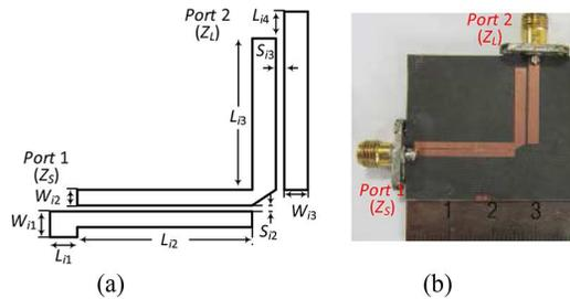
Fig. 4. (a) EM simulation layout and (b) photograph of fabricated PCB. ( $W_{i1} = 2.4$ ,  $L_{i1} = 2$ ,  $W_{i2} = 1.35$ ,  $L_{i2} = 22.7$ ,  $S_{i2} = 0.3$ ,  $W_{i3} = 2.4$ ,  $L_{i3} = 17.2$ ,  $S_{i3} = 0.65$ , and  $L_{i4} = 3$ ) (unit: mm).
