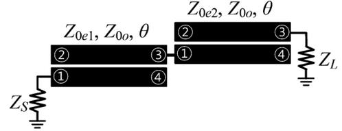
Fig. 1. Proposed circuit for ultra-high impedance transforming ratios.
