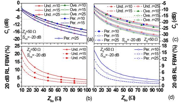
Fig. 3. Design graph according to  $Z_{0o}$  and different  $r$ : (a)  $C_1$ , (b) 20 dB return loss (RL) FBW of under-matched region, (c)  $C_2$ , and (d) 20 dB RL FBW of perfectly matched region.
