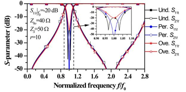
Fig. 2. Frequency responses of transformer for three different matched regions.
