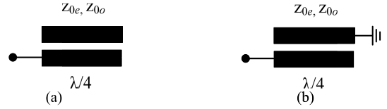
Fig. 2. Equivalent circuits of the proposed GD circuit type-I under (a) even- and (b) odd-mode excitations.
