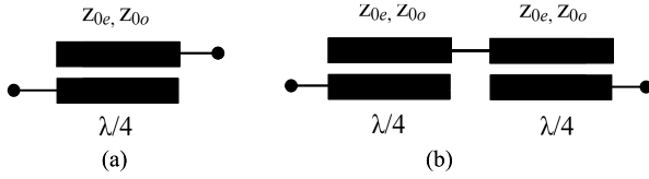
Fig. 1. (a) Coupled line and (b) proposed structure of wideband GD circuit type-I.
