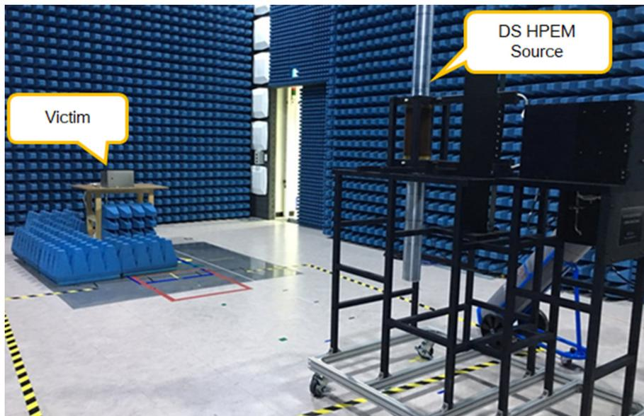
Fig. 6. DS HPEM source in anechoic chamber.
