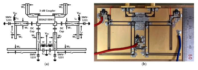
Figure 8. (a) Layout and (b) photograph of fabricated dual-band tunable reflection-type PS.
