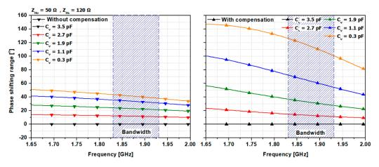
**Figure 5.** PSR with and without compensating for the effects of a of  $\lambda/4$  shunt open stub at the low–band.
