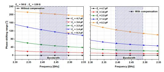
**Figure 7.** PSR with and without compensating for the effects of a  $\lambda/4$  shunt open stub at the high band.
