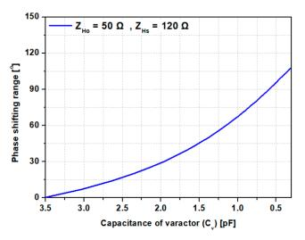
**Figure 4.** PSR with  $C_v$  variations at  $f_L$  ( $C_v = 3.5$  to 0.3 pF @ $f_L$ ).
