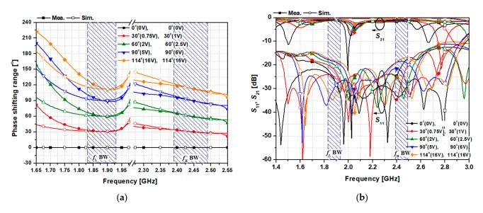
**Figure 11.** Simulated and measured results of a dual-band PS achieved by simultaneously varying the bias voltages of the low– and high–band: (**a**) PSR; (**b**) ILs and input/output RLs.
