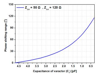
**Figure 6.** PSR with  $C_v$  variations at  $f_H$  ( $C_v = 4.7$  to 0.3 pF @ $f_H$ ).
