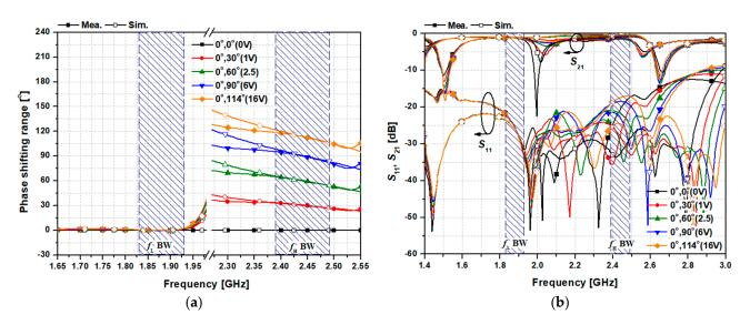
**Figure 10.** Simulated and measured results of a dual-band PS achieved by varying the bias voltage of the high—band while fixing the bias voltage of the low-band at 0 V: (**a**) PSRs; (**b**) ILs and input/output RLs.
