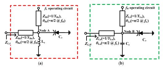
**Figure 3.** Each reflection load according to operating band: (**a**) Low-band operation; (**b**) High-band operation.
