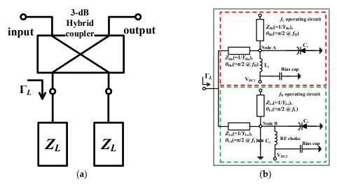
**Figure 1.** Structure of the proposed dual-band PS: (**a**) Overall two-port circuit using a 3-dB hybrid coupler and reflection loads; (**b**) One-port reflection load.
