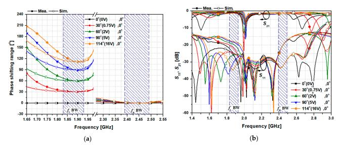
**Figure 9.** Simulated and measured results of a dual-band PS achieved by varying the bias voltage of the low—band while fixing the bias voltage of the high-band at 0 V: (**a**) PSRs; (**b**) ILs and input/output RLs.
